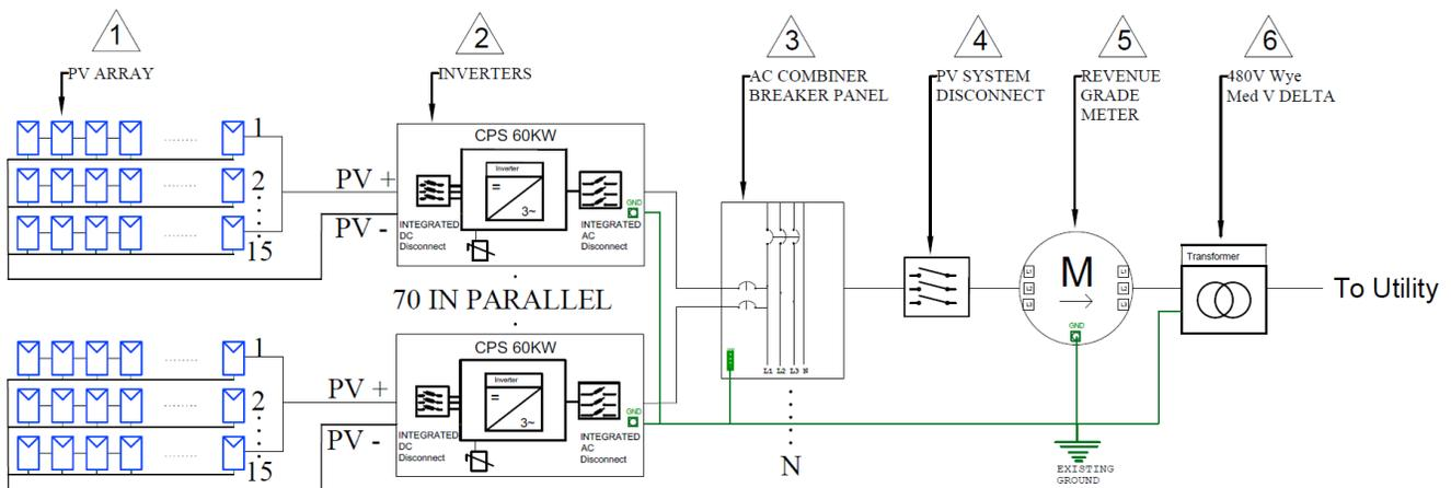
**Example: 4.2MW building block with 60kW inverters**
