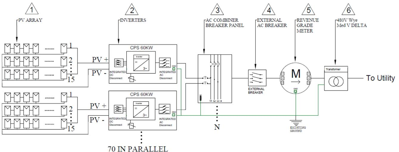
Example: 4.2MW building block with 60kW inverters
