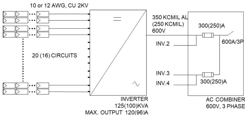
Figure 2.1.2. Configuration with Two Inverters per Circuit Breaker or Fuse
