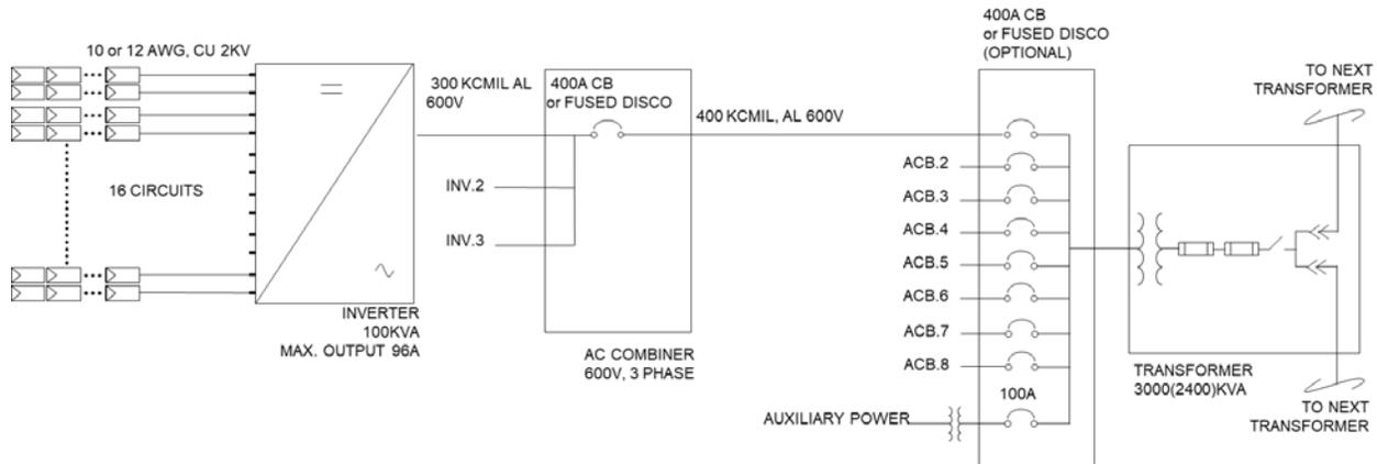
Figure 2.2.1. Configuration with Three Inverters to a 400A Fuse or Circuit Breaker
