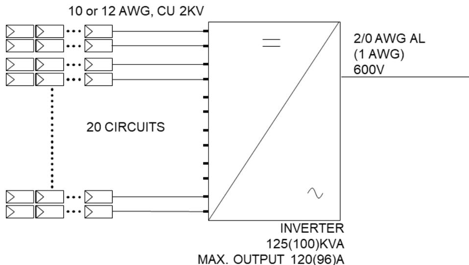
Figure 1.1. Configurations for One String per Input
