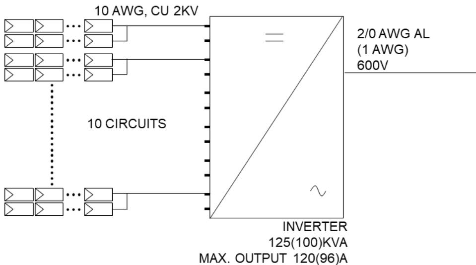
Figure 1.1. Configurations for Two-Strings per Input
