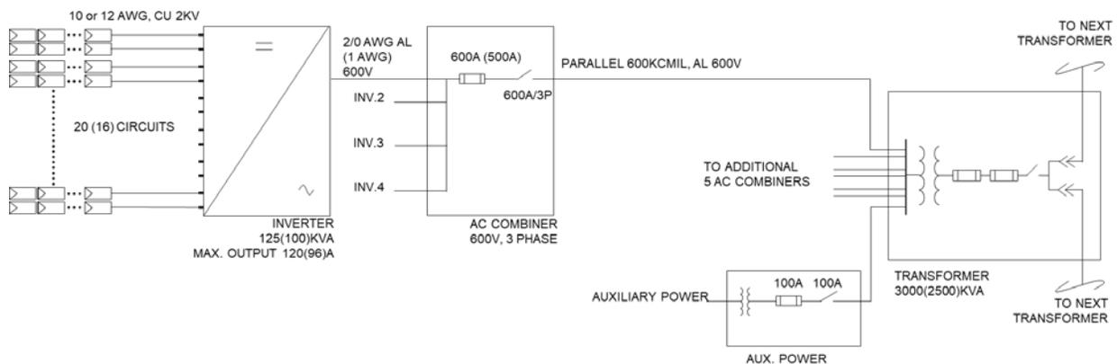
Figure 2.3.1 Four Inverter Cluster with 600A Fused Disconnect Connected Directly to Transformer
