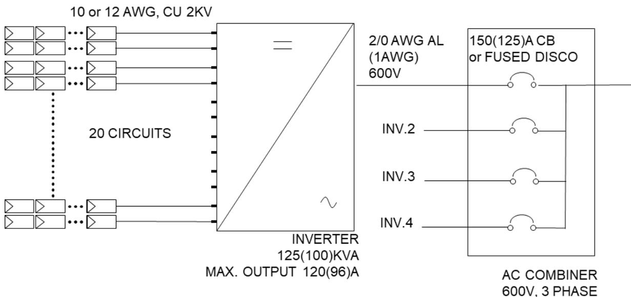
Figure 2.1.1. Configuration with One Inverter per Circuit Breaker or Fuse
