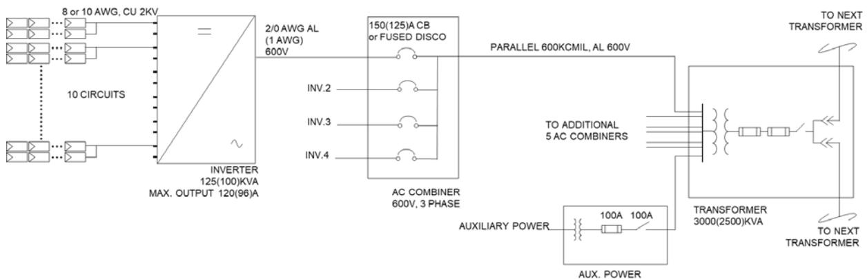
Figure 2.2.3 Configuration with Four Inverter Cluster Directly to Transformer
