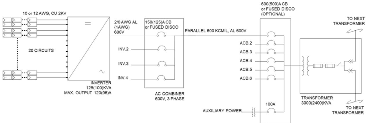
Figure 2.2.2. Configuration with Four Inverter Cluster to Switchgear
