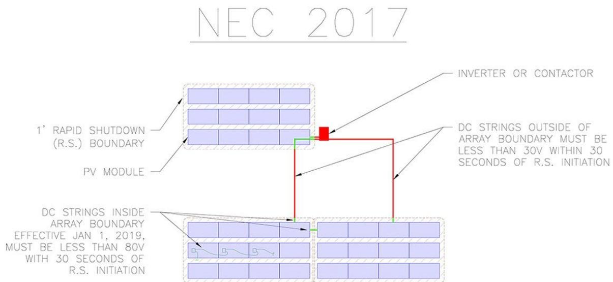
Figure 1: Example of a rapid shutdown-compliant array per NEC 2017 (source: [Pure Power Engineering](#))
